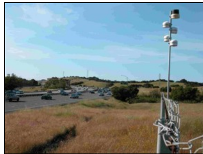
Figure 2. Ogawa passive samplers monitor pollutant concentrations at Edgewood Natural Preserve (San Mateo County, CA), where Highway 280 carries more than 100,000 vehicles daily.
